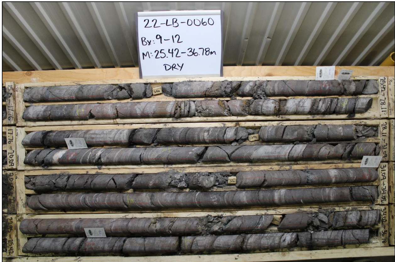
Figure 7—2: Core Photo of Oxide Facies from Project Drill Hole 22LB0060 (25.42 to 36.78 m)
