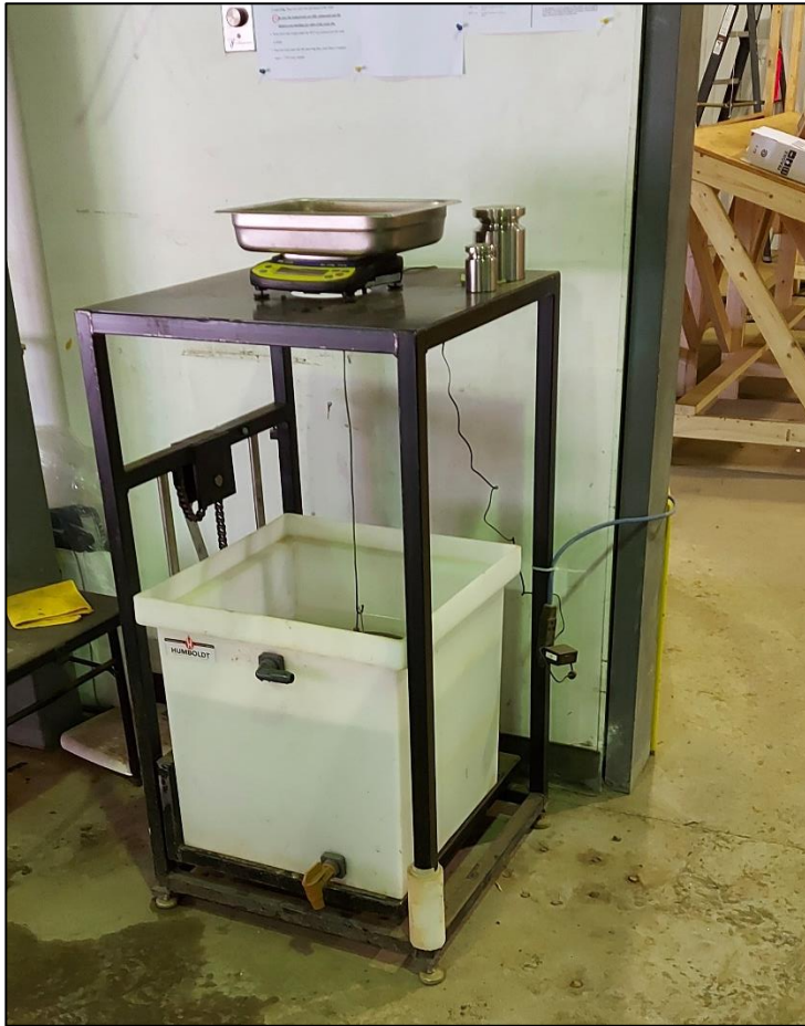
Figure 11—2: 2022 Water Immersion Specific Gravity Station
