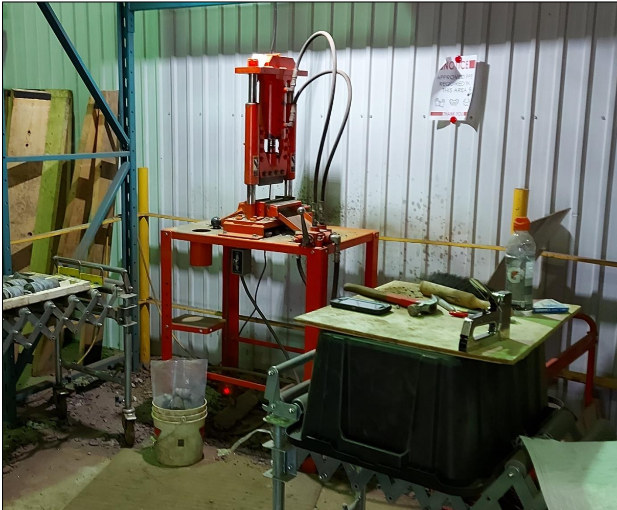
Figure 11—1: 2022 Core Splitter Setup
